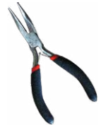
Pliers to break through a cable guide
